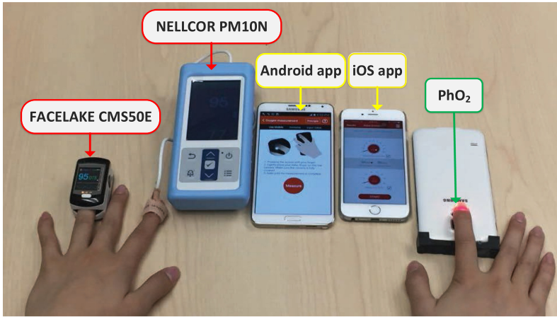
Fig. 11. Experiment setup to compare PhO 2 with other four pulse oximeters.
